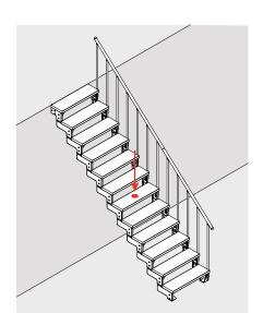
STAIR POINT LOAD Max. 2 kN ~ 200 kg
